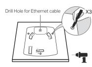
Place the mounting bracket in the center of the ceiling tile. Mark three positions for the screw holes and a position for the Ethernet cable hole.
