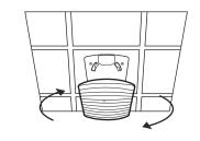
Connect the Ethernet cable to the ETHERNET port. Attach the EAP to the mounting bracket by aligning the arrow mark ▲ on the EAP with the arrow mark on the mounting bracket, then rotate the EAP until it locks into place, as shown on the
