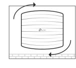
Attach the EAP to the mounting bracket by aligning the arrow mark ▲ on the EAP with the arrow mark ▲ on the mounting bracket, then rotate the EAP until it locks into place, as shown on the left.
